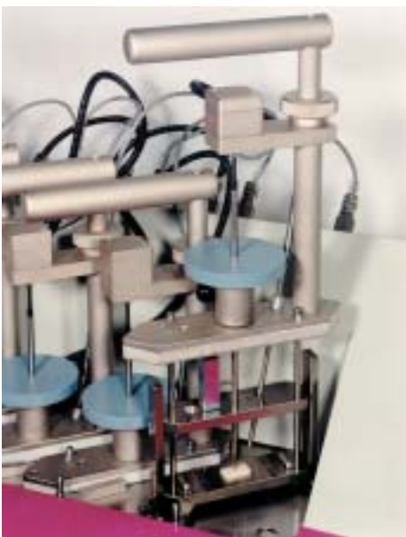
VICAT test station
